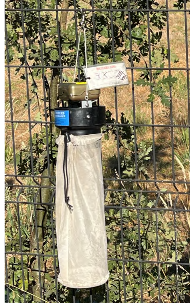
Traditional EVS trap with fan, light and catch bag
